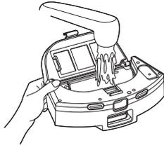
(6) Turn the tank over and remove mop for cleaning or replace it.
