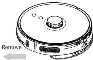
(2) Press the Dust Compartment release button to remove the 2-in-1 Dust Compartment with Water Tank.
