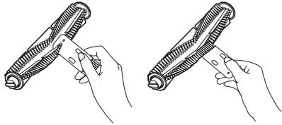
(3) Mount the main brush and main brush cover and lock the clamp.
