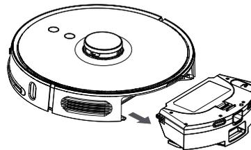
(2) Release the Dust Compartment clamp to remove filter screen clamp.
