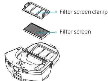
(4) Clean the filter screen and clamp with cleaning brush.
