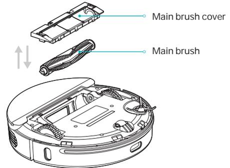
(2) Cut off hairs around the brush with knife, and clean the main brush with the other end of the knife.
